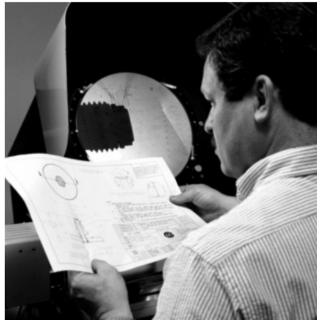
The Optical Comparator is used for small parts which are difficult to accurately measure by manual methods. Enlarged detail, vertical and horizontal measuring capabilities and profile projection allow the precise measurement of features such as radii, thread profile and angles.
